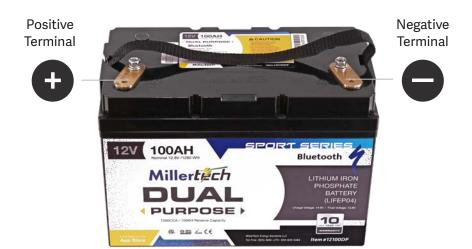
All batteries ship with 18-8 stainless steel M8 bolts/washers. If multiple lugs are used the washers may be removed, or longer bolts may be required in order for the bolt to fully seat into the copper pillar.
